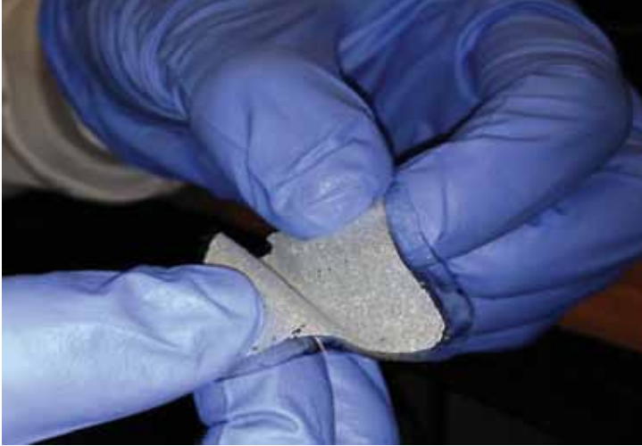
Figure 2 | A highly flexible, air stable, printed Zinc Poly battery cell
