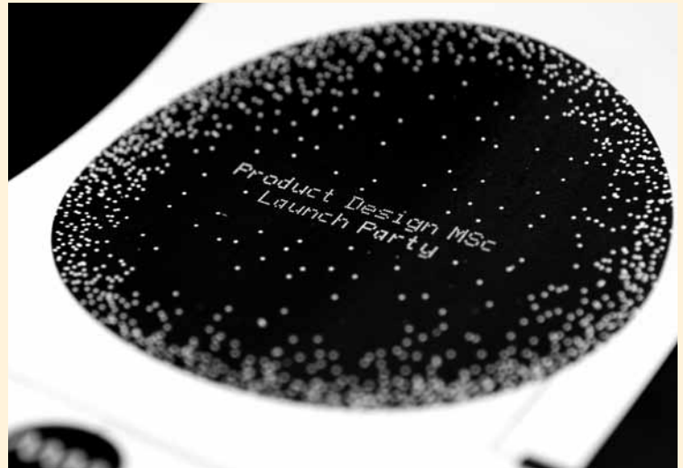
Figure 3 | An interactive invitation using screen-printed Bare Paint as a capacitive sensor. Touching the various images triggers and modulates sounds.
