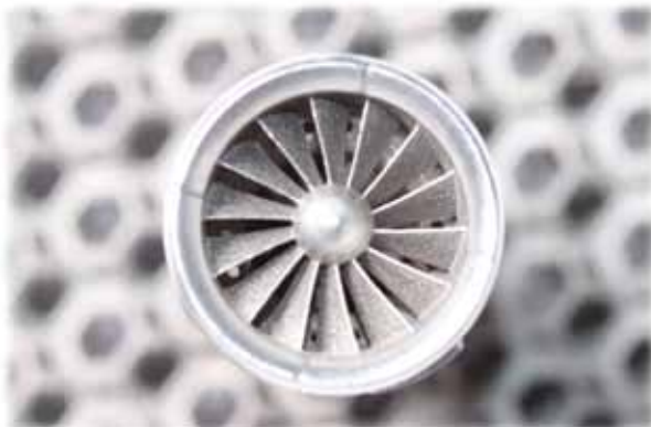
Figure 2 | Miniature turbine manufactured using Direct Metal Laser Sintering
