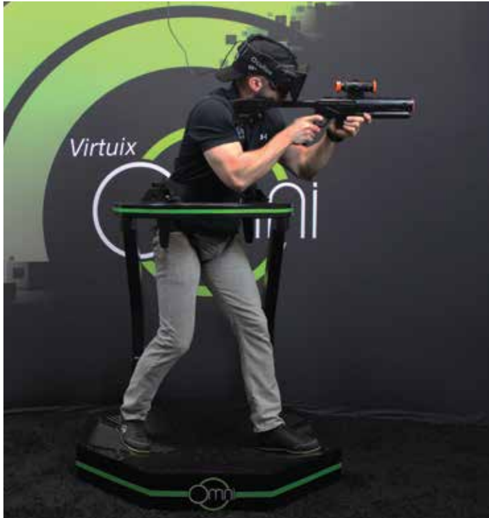
Figure 3 | The Virtuix Omni is an omnidirectional treadmill that allows the user to walk, run, jump, and interact within a 360-degree virtual environment.
