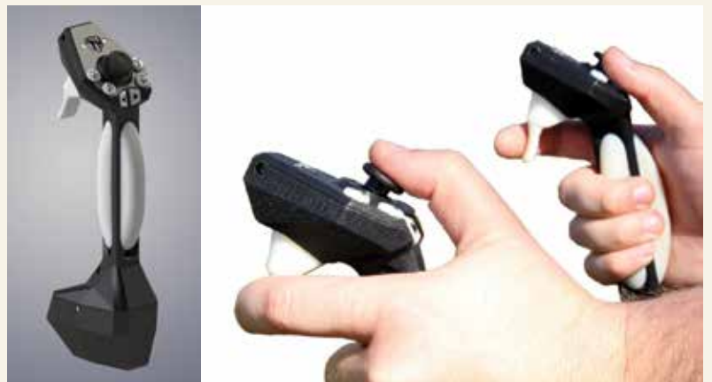
Figure 1 | Tactile feedback device with sliding contactor plates placed around the handle. The contactor plates are independently actuated and slide vertically.
