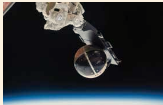
Figure 1 | (Left) The Dragon capsule unloads the SpinSat container, marking the first time an energetic material (rocket propellant) has ever been allowed inside the ISS. (Right) The SpinSat satellite before its release from the Cyclops deployer outside the International Space Station. (Photo: NASA)
