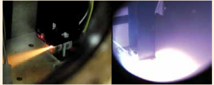
Figure 2 | Identical DSSP microthrusters burning in chemical mode ( left ) and electric mode ( right ), exhibiting characteristic purple “glow discharge” from plasma formation.
