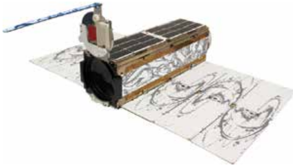
Figure 1 | The Planet Labs Dove spacecraft (3U form factor).
